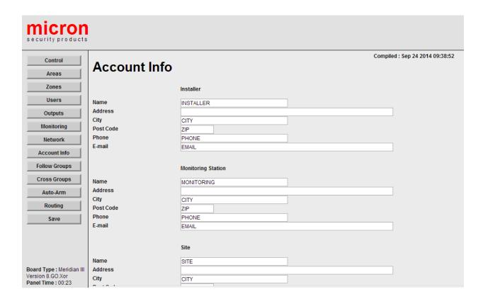
The Installer Name, Monitoring Station and Site details can be entered in this page.
